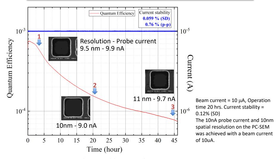
SEM imaging during stable  $10\mu A$  e-beam.
